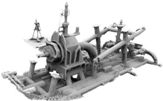
COMEX ORUS 3D (3000m) subsea metrology system for Oil&Gas industry
